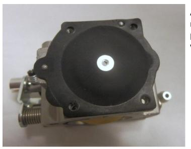
After the main membrane is in place, close it with its cover
