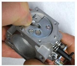
Insert again the rocker arm, tighten the screw and reclose the carburetor with the main membrane cover
