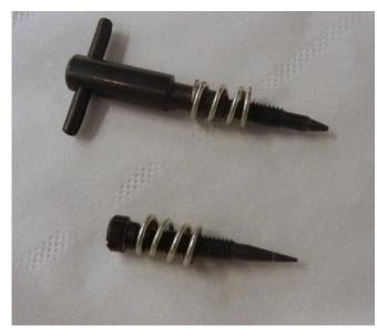
Check that the tips and bodies of the H and L screws are not damaged or bent. Reinstall the screws closing them completely, and make the proper carburation again. Standard carburation is 40 minutes for the L screw and 1 turn and 35 minutes for the H screw
